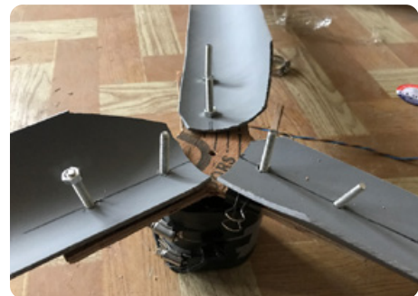
Figure 10: Blade attachment to generator
