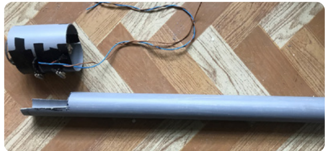
Figure 5: L shape cut out from tail boom for generator; Slit on the tail boom for tail fin
